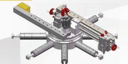
FI2000 Flange Facing Machine adopts the disk type slewing bearing support structure, relative to the spindle structure, the anti-overturning moment of the equipment is enhanced, and the overall height of the equipment is greatly reduced, especially the seismic ability of the tool arm is enhanced during vertical processing.
